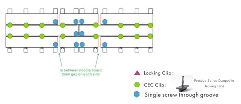
\*\*Note: Always pre-drill when nailing/screwing into the boards for the best results. Never use 2 Locking clips on one board.
