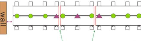
in between middle board: 2mm gap on each side
