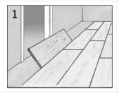
Some long edge joints cannot be installed using a  $20^{\circ}$  angle.
