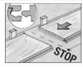
Lay panels close together on the floor.
