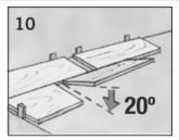
Lock in panel lengthwise. Allow 12" minimum end-joint stagger row to row.
