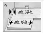
Observe 3/8" clearances for expansion and 16" minimum for smallest usable piece.
