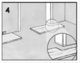
If possible, start to lay panels under the door jam and finish installing planks on a wall without a door jam. See "Working with Limited Clearance" section.
