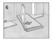
Remove the tongue on the panels that face the walls to allow room for spacers and prevent problems from spills.
